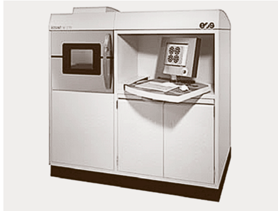
Fig. 7.334 EOSINT M270 – EOS device. Technical characteristics: materials: tool steel H20, steel DS20, Ti6AL4V, stainless steel EOS 17-4 PH, bronze DM20; full melting; layer thickness 20–100 μm; accuracy 0.05–0.1 mm; build volume 250 × 250 × 215 mm; speed 5–70 cm 3 /h
