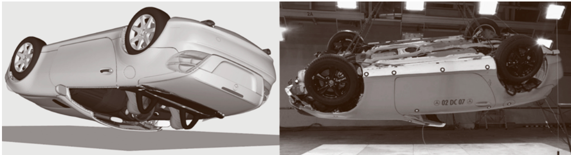
Fig. 13.66 Crash simulation and hardware crash of a convertible (courtesy of Mercedes Car Group)
