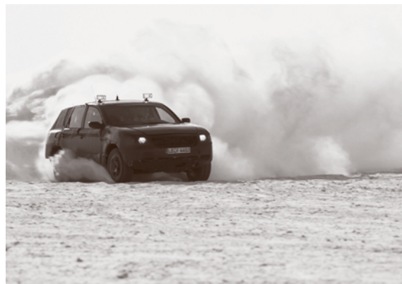
Fig. 13.82 Test with sports utility vehicle to verify performance in cold and snow environment (courtesy of Dr. Ing. h.c. F. Porsche AG)
