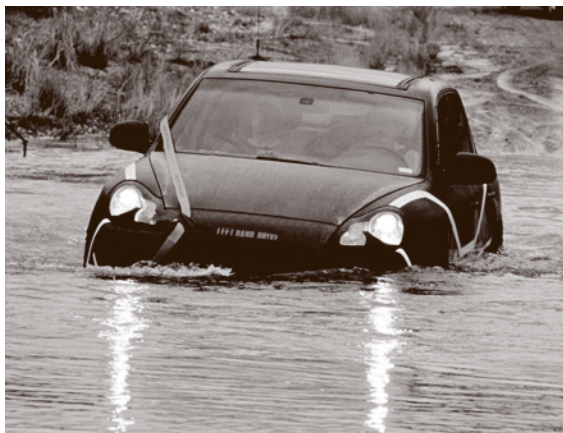
Fig. 13.83 Test with sports utility vehicle to verify performance in wet environment (courtesy of Dr. Ing. h.c. F. Porsche AG)
