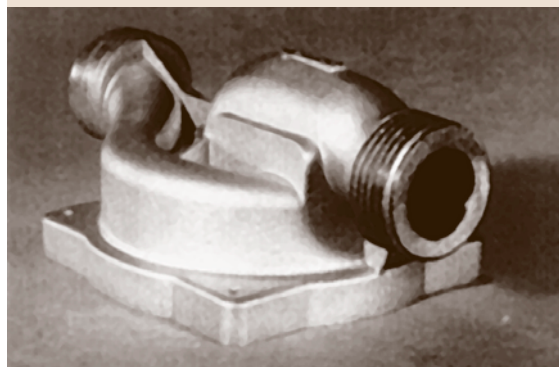
Fig. 7.326a,b Diagram of model manufacture by SLS method (a) and a model prepared this way (b)
